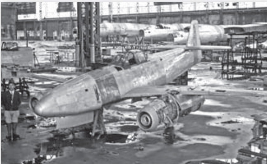
The Nakajima Kikka (Orange Blossom) was patterned after the German Me-262, but was somewhat smaller. There was controversy over its intended use, with some navy commanders urging its application as a fast bomber, even though it was nominally part of the Tokko aircraft program. It flew only once prior to war's end, due to delays with the associated Ne-20 turbojet engine effort. (NARA)
