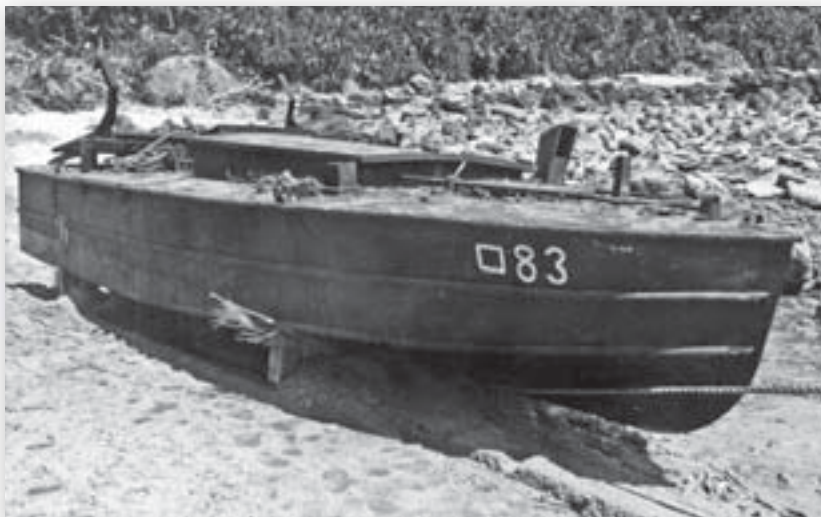
The army Renraku-tei boats can be distinguished from the navy Shinyo by the claw-shaped rack on the stern on either corner, which carried the boat's depth charge. This particular boat was captured on Aka Shima during the Okinawa campaign. (NARA)
