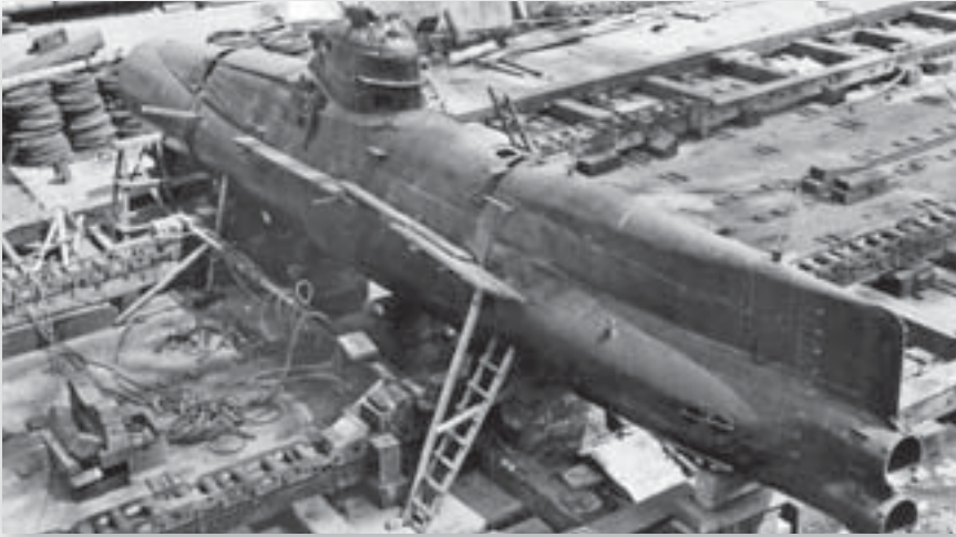
One of the more common Tokko submarines was the Koryu Type D; there were plans to complete 570 by the end of September 1945 at the Yokosuka navy yard. It had a crew of five and was armed with two 45cm torpedoes stacked one atop each other in the bow. (NARA)
