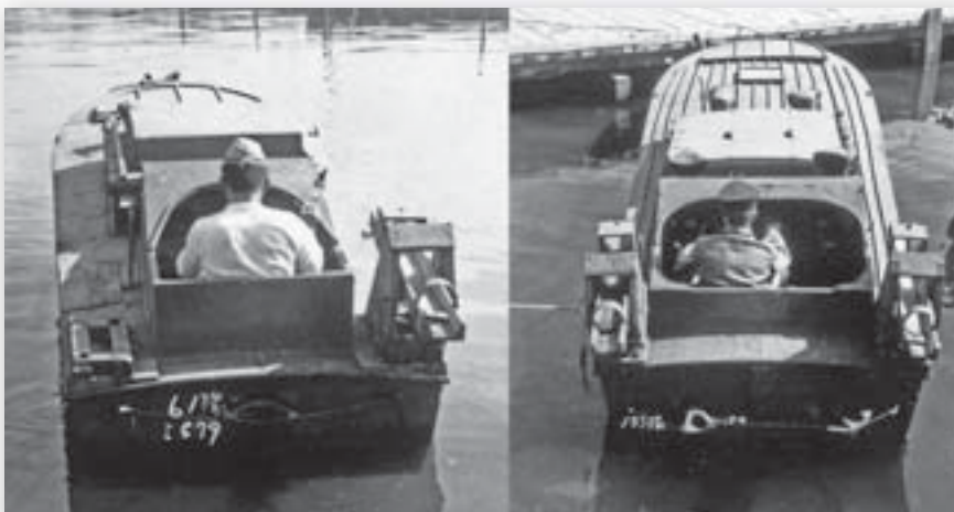
This comparison photo from the stern shows the difference between the Type 1 (left) and Type 5 (right) Shinyo boats. The Type 1 had a single pilot while the Type 5 had a crew of two with a second sailor manning the 13mm machine gun. (NARA)
