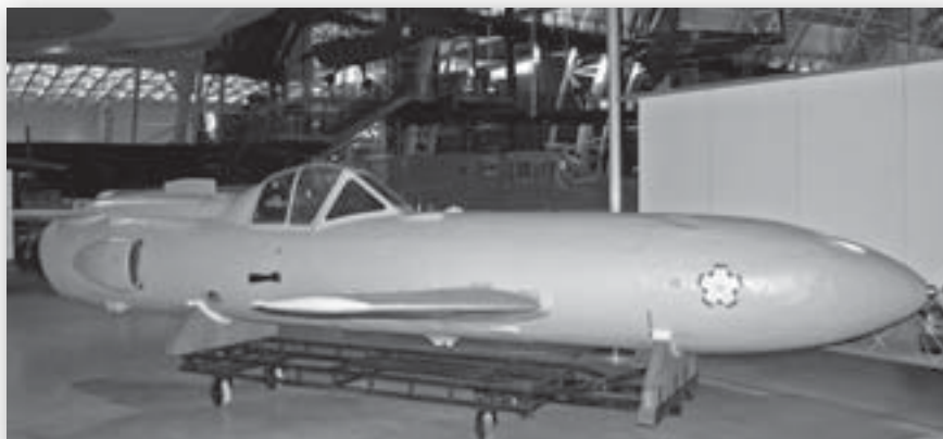
The Ohka Model 22 did not enter service due to problems with its engine. This example was restored at the Udvar-Hazy Center at the US National Air & Space Museum. (Author)
