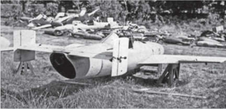
The final production batches of Ohka aircraft had a metal fairing at the rear of the cockpit canopy, instead of the clear section on the earlier production run. This particular example was part of an Ohka unit being stored at Kawaya near Nagasaki at the end of the war. (NARA)
