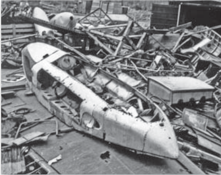
One of the lesser-known Tokko modification efforts was the development of this ventral fairing for modifying light bombers for kamikaze missions. It was designed to carry a 1,760lb (800kg) warhead, and had special fittings for four booster rockets to accelerate the aircraft during the terminal dive. (NARA)
