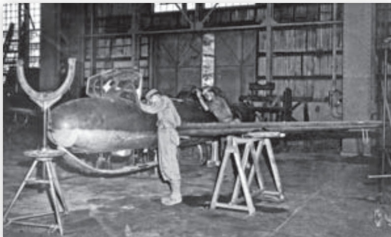
The Ohka K2 trainer was the only version of the Model 43 to enter production and can be distinguished both by its twin canopy configuration but also by the extended wings. This particular example was found at the Kugisho facility in Yokosuka at the end of the war. (NARA)
